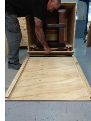
Step 2: Place the lid on the corner of the pallet with the supports prepared for it, and lower the link with the ramp.
