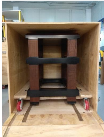
Step 3: Remove the table carefully and place it in the final place where it will be installed
